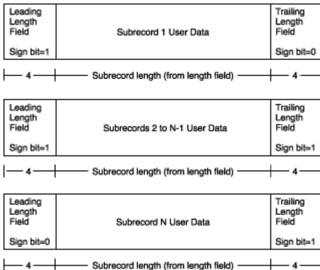
Files written with variable-length records by Intel Fortran programs usually cannot be accessed as text files. Instead, use the Stream\_LF record format for text files with records of varying length.
