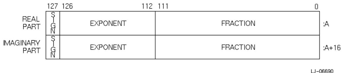
The limits and underflow characteristics for [REAL\(16\)](#) apply to the two separate real and imaginary parts of a [COMPLEX\(16\)](#) number. Like [REAL\(16\)](#) numbers, the sign bit representation is 0 (zero) for positive numbers and 1 for negative numbers.
