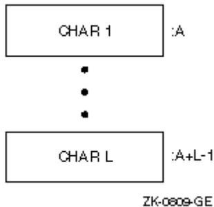
A character string is specified by two attributes: the address  $A$  of the first byte of the string, and the length  $L$  of the string in bytes. The length  $L$  of a string is in the range 1 through 2,147,483,647 ( $2^{31}-1$ ).
