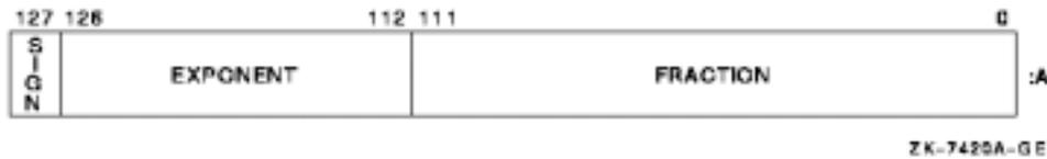
The form of REAL(16) data is sign magnitude, with bit 127 the sign bit (0 for positive numbers, 1 for negative numbers), bits 126:112 a binary exponent in excess 16383 notation, and bits 111:0 a normalized 113-bit fraction including the redundant most-significant fraction bit not represented.
