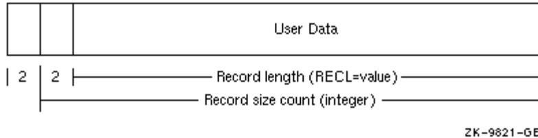
The control information consists of a 2-byte integer record size count (includes the two bytes used by the segment identifier), followed by a 2-byte integer segment identifier that identifies this segment as one of the following:
