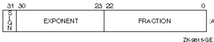
The form of REAL(4) data is sign magnitude, with bit 31 the sign bit (0 for positive numbers, 1 for negative numbers), bits 30:23 a binary exponent in excess 127 notation, and bits 22:0 a normalized 24-bit fraction including the redundant most-significant fraction bit not represented.
