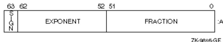
The form of REAL(8) data is sign magnitude, with bit 63 the sign bit (0 for positive numbers, 1 for negative numbers), bits 62:52 a binary exponent in excess 1023 notation, and bits 51:0 a normalized 53-bit fraction including the redundant most-significant fraction bit not represented.
