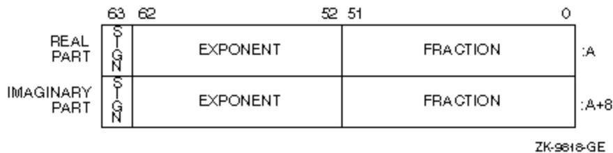
The limits and underflow characteristics for [REAL\(8\)](#) apply to the two separate real and imaginary parts of a [COMPLEX\(8\)](#) number. Like [REAL\(8\)](#) numbers, the sign bit representation is 0 (zero) for positive numbers and 1 for negative numbers.
