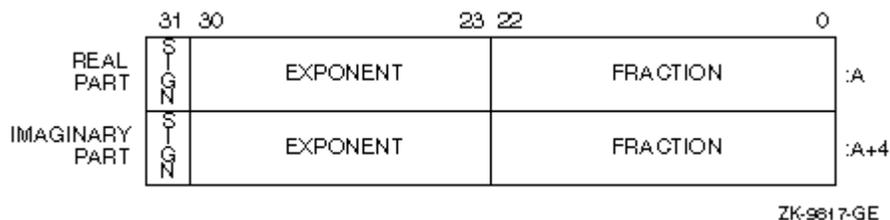
The limits and underflow characteristics for [REAL\(4\)](#) apply to the two separate real and imaginary parts of a [COMPLEX\(4\)](#) number. Like [REAL\(4\)](#) numbers, the sign bit representation is 0 (zero) for positive numbers and 1 for negative numbers.
